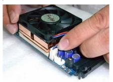
Connecting the fan's power cable to the *PL-P3/SMP*.
